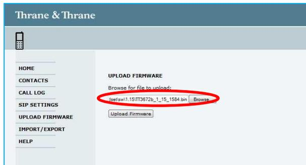
5. Choose **Upload Firmware** and verify that the upload is in progress as shown below (status bar enabled in browser).
