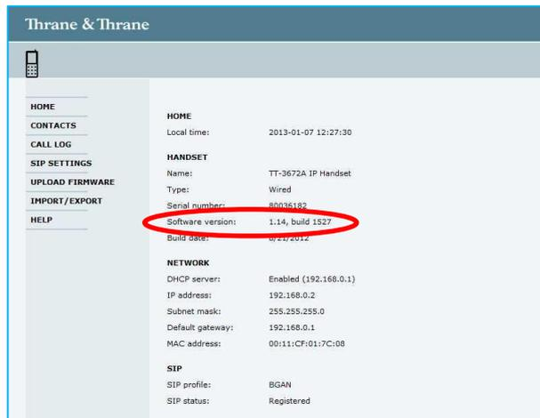
2. If using a FleetBroadband Terminal: Open your web-browser, on the PC /Laptop, and open the Web Interface of the IP Handset. The IP address can be found in the Thrane IP Handset menu **Status** → **Network Information**.
