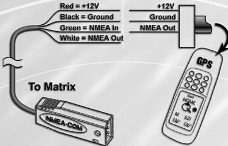
**Caution!** Please use caution before connecting the red +12V wire to your handheld GPS receiver, and consult your handheld GPS receiver manufacturer's user manual before connecting power and ground, as some handheld GPS receivers have a different voltage input than 12V.
