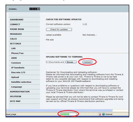
**13.** The terminal will reboot. When all terminal LEDs are lit green and the upload is complete, access the web interface again (192.168.0.1) and verify the Dashboard shows the new software version. Also make sure no new warnings appear in the Event List.
