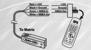
**Caution!** Please use caution before connecting the red +12V wire to your handheld GPS receiver, and consult your handheld GPS receiver manufacturer's user manual before connecting power and ground, as some handheld GPS receivers have a different voltage input than 12V.
